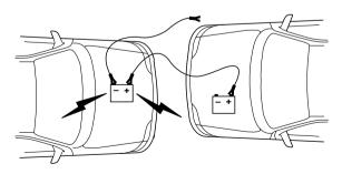
2. Remove the jumper cable on the negative (-) connection of the booster vehicle's battery.
